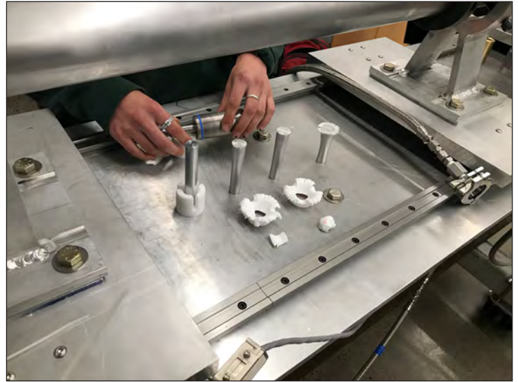
Figure 3. Sabot and aluminum Taylor cylinders in unfired and fired configurations, at higher velocities from left to right.
