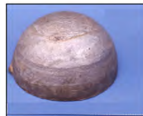
Cast aluminum hemisphere
