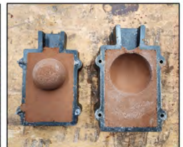
3D printed match plate and sand filled casting flask
