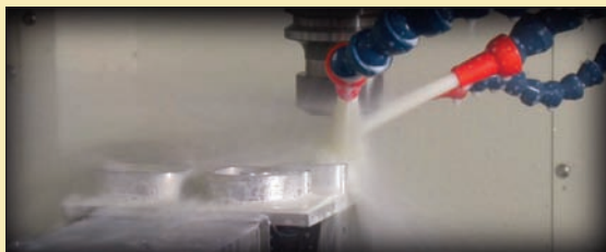
A cutting solution also cools and washes particles away during the precision machining process.
