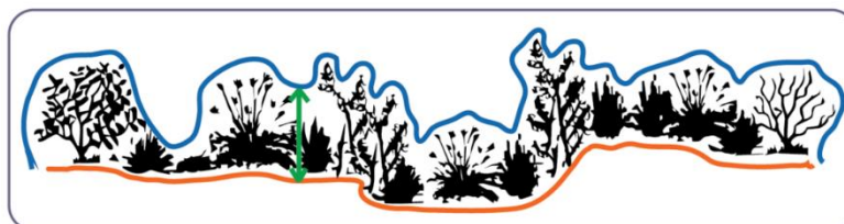
Figure 4. Subtracting the DSM from the DTM yields canopy height estimates (Fig 5B)
