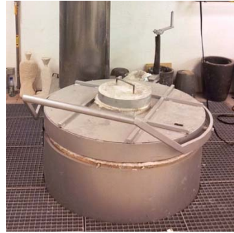
Example of furnace (indicative, installed in pit)
