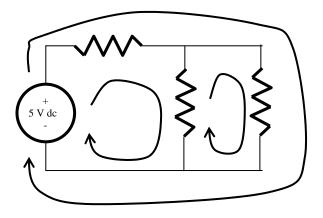
A *branch* is a path from one node to an adjacent node. A circuit branch contains one or more components (resistors, capacitor, etc.).
