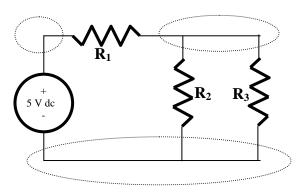
A *loop* is a connected path through a sequence of elements that starts and ends at the same node without crossing itself. A circuit must have at least one loop. If there is more than a single loop, the separate loops of a circuit generally partially overlap one another.
