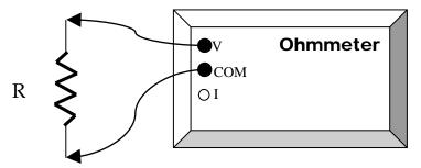
Although an "ideal" voltmeter would act like an open circuit (no current through the meter) and an ideal ammeter would act like a short circuit (no voltage across the meter), the instruments actually available for these measurements cannot be perfect. This means that the multimeter may actually *load* the circuit being measured by changing the resistance between the test points. This problem is particularly important when measuring circuits with resistances comparable to the meter resistance.
