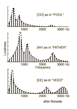
Signal rich in harmonics (a "buzz") with spectral shaping
