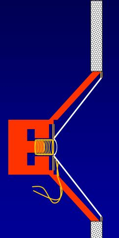
Baffle prevents front-back interaction: improved low frequency performance
