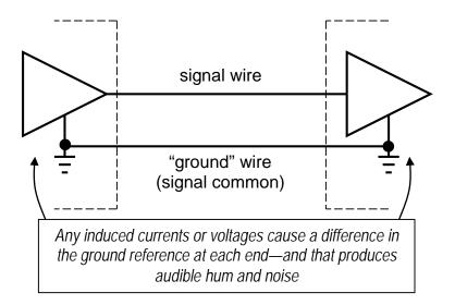
Unbalanced connections are inexpensive and work reasonably well for consumer devices that are located close to each other, like a stack of gear in a stereo cabinet. However, the unbalanced connection is susceptible to both electric field pickup and magnetic field coupling.
