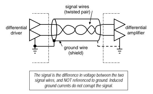
Most professional audio gear is designed with balanced interconnections in mind. Most consumer gear (and even most "audiophile" stereo and a/v equipment!) uses unbalanced
