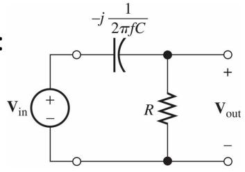
• Low frequencies are blocked, high frequencies are passed through to  $v_{\text{out}}$
