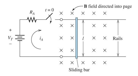
Force on sliding bar due to current =  $i_A \mathbf{I} \times \mathbf{B}$
