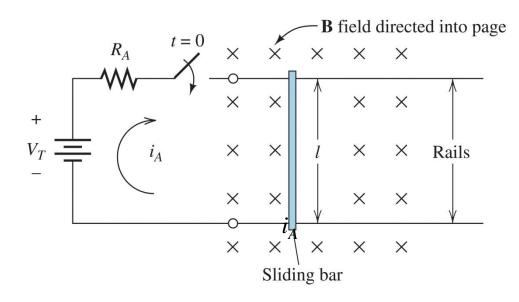
At t = 0, bar is at rest, and initial current  $i_{A0} = V_T / R_A$ At t = 0, initial force on bar is  $i_{A0} l B$  to the right
