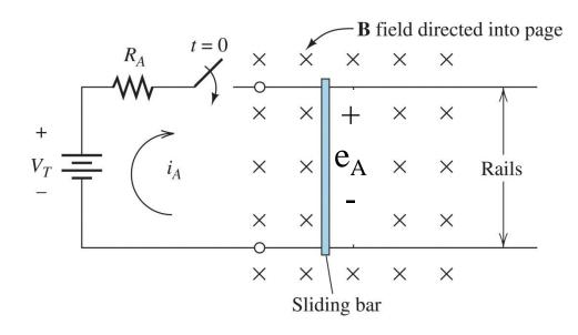
As bar accelerates due to force, the voltage  $e_A$  across the bar increases as its velocity *u* increases: B *l u*
