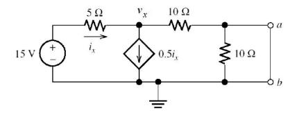
$i_x=\frac{15-v_x}{5}$   $\frac{v_x}{10}-i_x+0.5i_x=0$  Solving, we find  $v_x=7.5\,\mathrm{V}$  and then we have  $i_{sc}=\frac{v_x}{10}=0.75\,\mathrm{A}$ . Then, we have  $R_t=v_{oc}/i_{sc}=6.67\,\Omega$ . Thus the equivalents are:
