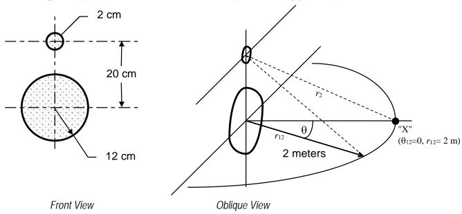
Each driver is modeled as a baffled piston radiator (<u>far field case</u>, K&F eqn. 7.4.17). Both drivers are operated at  $\mathbf{f} = \mathbf{5} \, \mathbf{kHz}$  into air at 20°C. The observation point is "X", located in the plane of the 12 cm driver.
