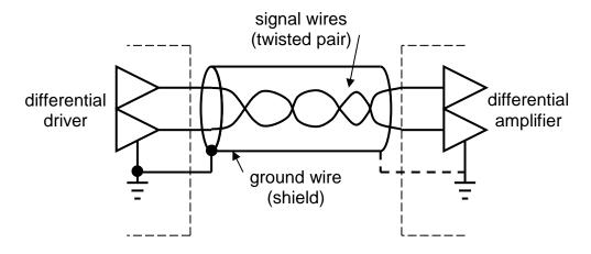
The signal is the difference in voltage between the two signal wires, and NOT referenced to ground. Induced ground currents do not corrupt the signal.
