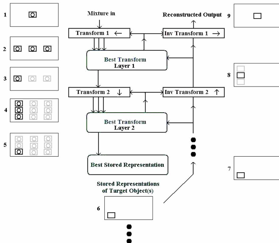
**Figure 1: MSC Configured to Find a Square in a Mixture.**
