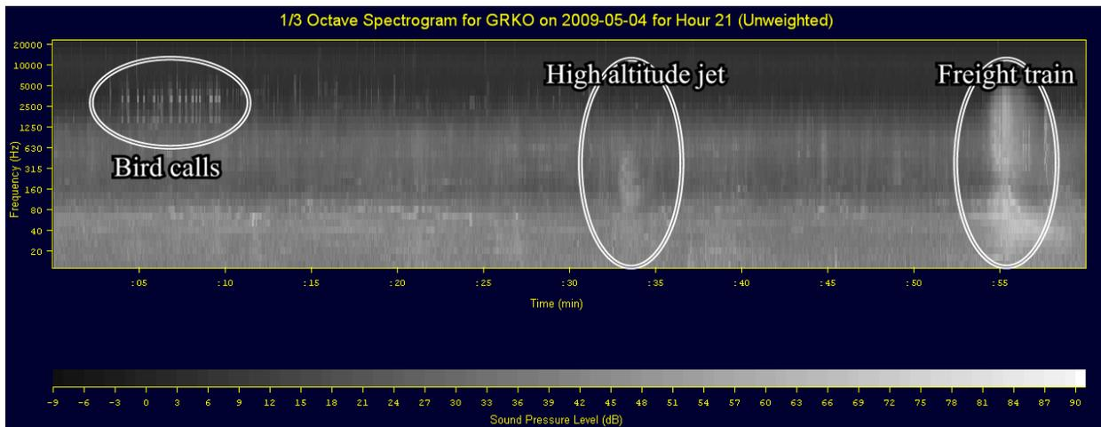
Figure 8: Example display showing the 1/3<sup>rd</sup> octave spectrogram for one hour of sound
