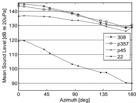
Figure 5: Comparison of mean sound pressure level for the 308 rifle, 357 and 45 pistols, and the 22 rifle, as a function of horizontal azimuth.
