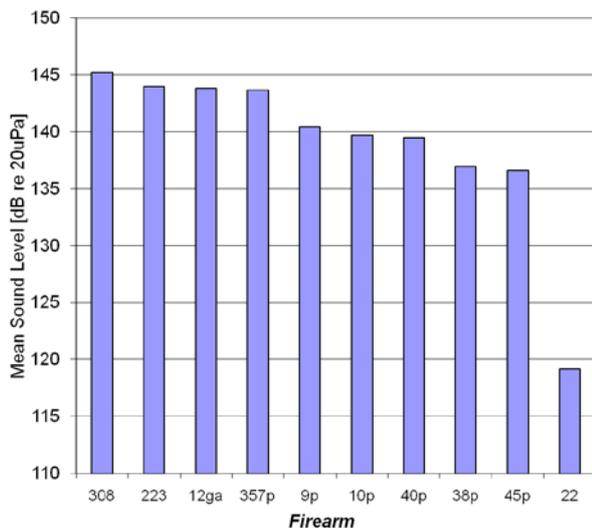
Figure 6: On-axis (max) mean SPL for ten firearms.
