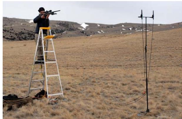
Figure 1: Example test configuration for firearm acoustical tests. The microphones are repositioned between shots to cover the 180 degree azimuth range.
