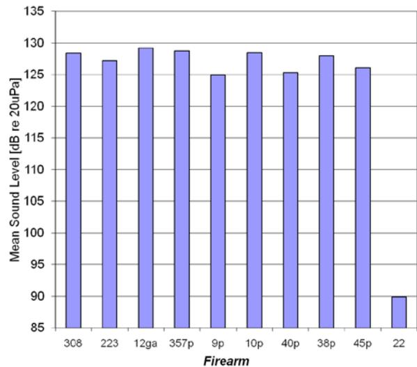
Figure 7: Minimum mean sound pressure level (off-axis) for ten firearms.
