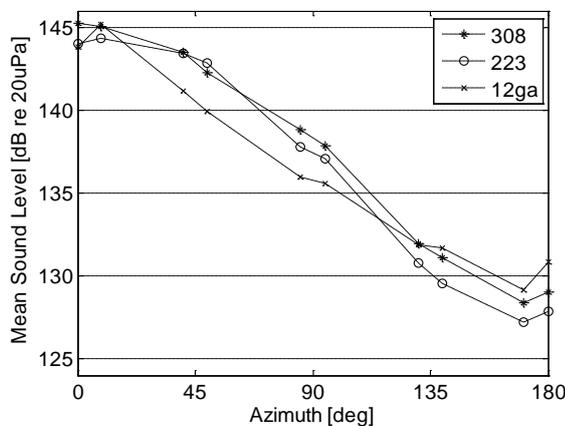
Figure 2: Comparison of unweighted mean SPL for the 308 and 223 rifles and the 12 gauge shotgun, as a function of horizontal azimuth.
