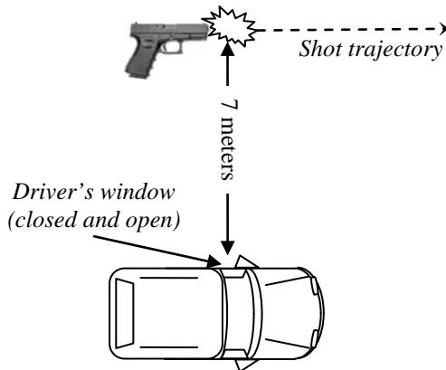
Figure 6: Experimental configuration for external gunshot recorded inside a parked vehicle.
