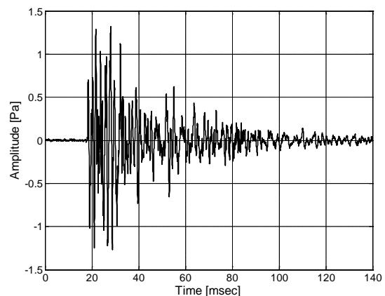
Figure 7: Recording of single gunshot, Glock 19 handgun, 9 mm ammunition. 24-bit, 48 kHz PCM, professional microphone inside closed vehicle, 7 meters from shooting position, 90° off-axis.
