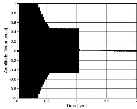
Figure 5: Response of digital voice recorder to 500Hz tone burst. Initial clipping with automatic gain reduction attack requiring 0.5 seconds, and approximately 1 second gain reduction release.
