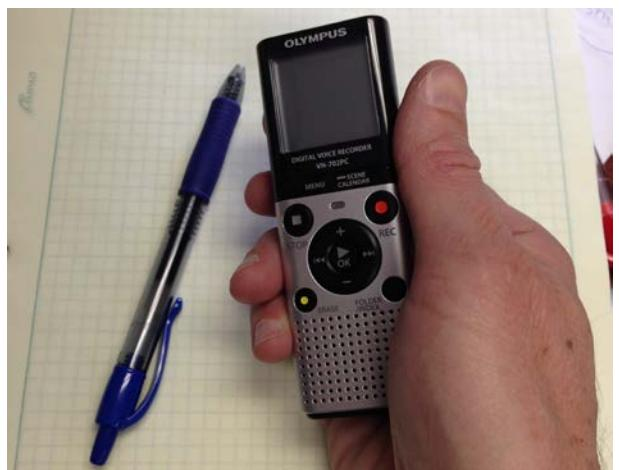
Figure 3: Example consumer digital voice recorder used in the tests: Olympus brand, model VN-702PC.
