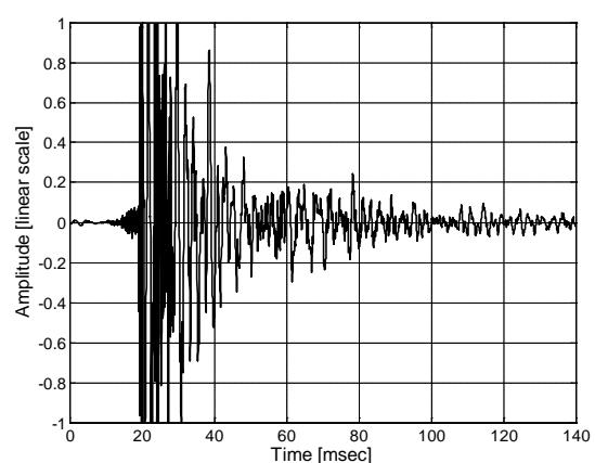
Figure 8: Recording of single gunshot, Glock 19 handgun, 9 mm ammunition. MP3, consumer digital voice recorder with built-in microphone inside closed vehicle, 7 meters from shooting position, 90° off-axis.
