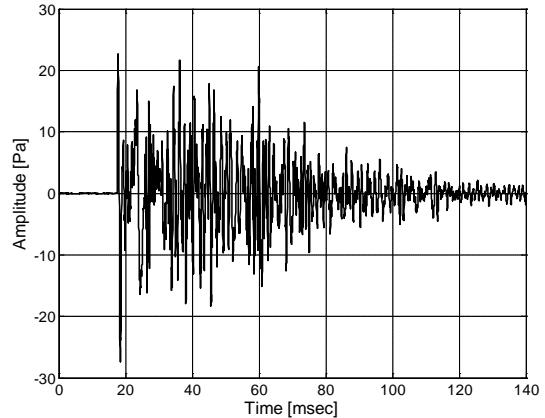
Figure 2: Reverberant recording of single gunshot, Glock 19 handgun, 9 mm ammunition. 24-bit, 48 kHz PCM, professional microphone at 8 meters, 90° off-axis.
