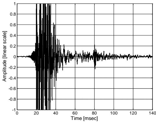
Figure 10: Recording of single gunshot, Glock 19 handgun, 9 mm ammunition. MP3, consumer digital voice recorder with built-in microphone inside open vehicle, 7 meters from shooting position, 90° off-axis.
