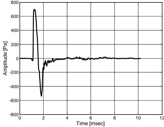
Figure 1: Anechoic recording of single gunshot, Glock 19 handgun, 9 mm ammunition. 24-bit, 48 kHz PCM, professional microphone at 3 meters, 9° off-axis.
