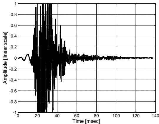
Figure 4: Reverberant recording of single gunshot, Glock 19 handgun, 9 mm ammunition. MP3, consumer digital voice recorder with built-in microphone at 3 meters from shooting position, 9° off-axis.
