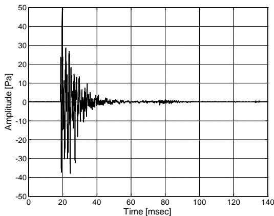
Figure 9: Recording of single gunshot, Glock 19 handgun, 9 mm ammunition. 24-bit, 48 kHz PCM, professional microphone inside open window vehicle, 7 meters from shooting position, 90° off-axis.
