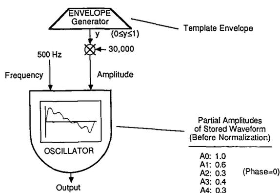
Fig. 12. Example synthesis algorithm comprising fixed-frequency, fixed-waveform oscillator with amplitude modulation applied by envelope generator.
