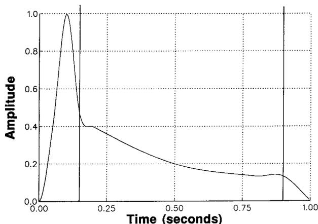
Fig. 18. Example template envelope (used in algorithm of Fig. 16) divided into three segments of durations (0.15, 0.75, 0.1) s.
