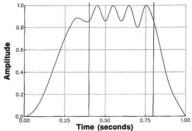
Fig. 13. Example template envelope (used in algorithm of Fig. 11) divided into three segments of durations (0.4, 0.4, 0.2) s.
