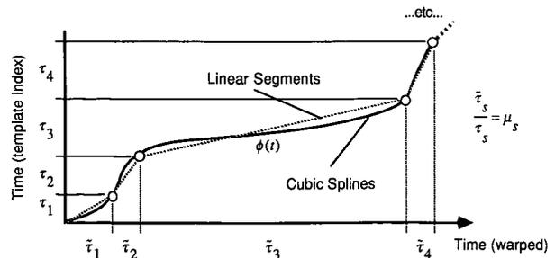
Fig. 9. Envelope lookup phase function represented as a concatenated set of smooth cubic-spline functions with matched slopes at each segment endpoint.
