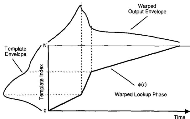
Fig. 7. Time-warped envelope produced from template envelope using nonlinear lookup function, denoted by  $\phi(t)$ . Unwarped envelope would be generated if  $\phi(t)$  were a straight line with slope 1.
