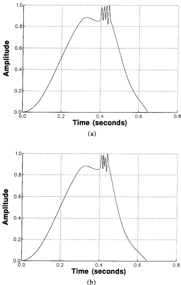
Fig. 15. Envelope of Fig. 12 compressed in overall duration to 0.65 s by time scaling sustain (middle) portion. (a) Compression using linear-segment lookup function. (b) Compression using cubic-spline lookup function.
