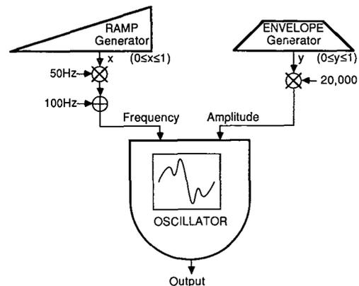
Fig. 4. Block diagram of simple synthesis algorithm: a fixed-waveform oscillator is amplitude modulated by an envelope generator and frequency modulated by a linear ramp function. Maximum output amplitude is 20 000 units; frequency varies from 100 to 150 Hz.
