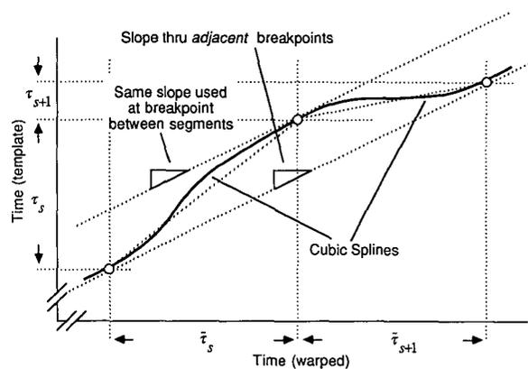
Fig. 10. Slope of phase function at segment boundaries within table can be chosen parallel to a line connecting two adjacent break points. This helps confine behavior of cubic splines between break points.
