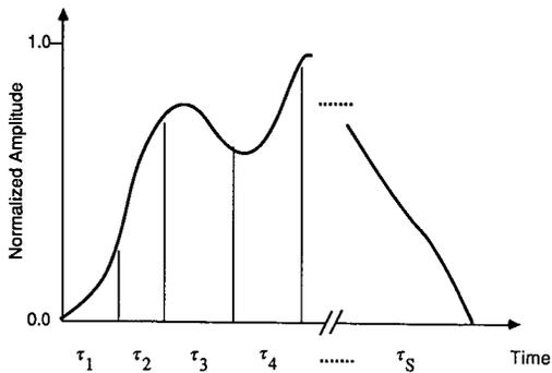
Fig. 8. Envelope function divided into  $S$  nonoverlapping sections. Each segment has a particular duration, denoted by  $\tau_s$ .
