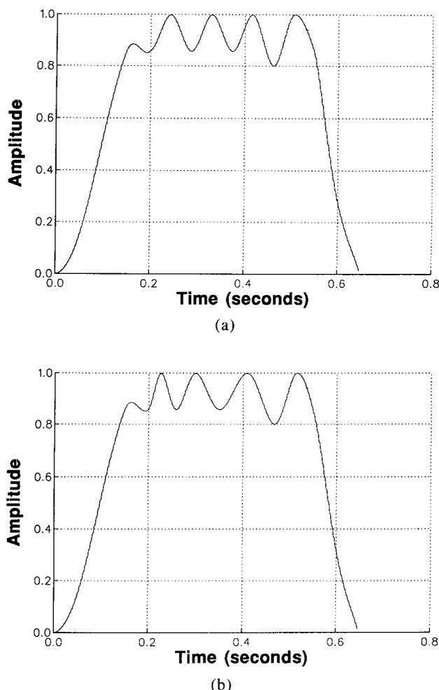
Fig. 16. Envelope of Fig. 12 compressed in overall duration to 0.65 s by time scaling all three segments by factors (0.5, 0.875, 0.5). (a) Compression using linear-segment lookup function. (b) Compression using cubic-spline lookup function.
