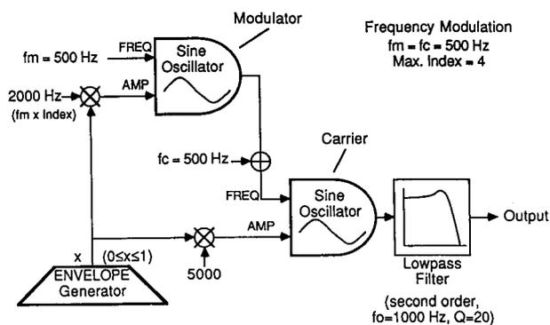
Fig. 17. Frequency modulation (FM) synthesis algorithm using modulation index, amplitude envelopes, and low-pass filter.
