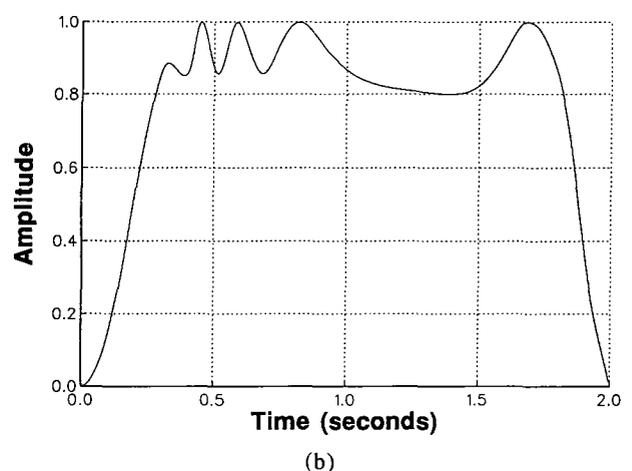
Fig. 14. Envelope of Fig. 12 expanded in overall duration to 2 s by time scaling sustain (middle) portion. (a) Expansion using linear-segment lookup function. (b) Expansion using cubic-spline lookup function.
