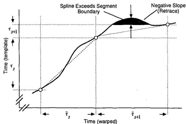
Fig. 11. Certain combinations of segment durations and time-warping factors may generate unacceptable lookup function which goes beyond end of desired envelope segment or retraces part of template. This situation must be detected and corrected.
