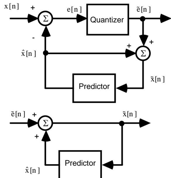
Figure 1: Basic DPCM structure.
