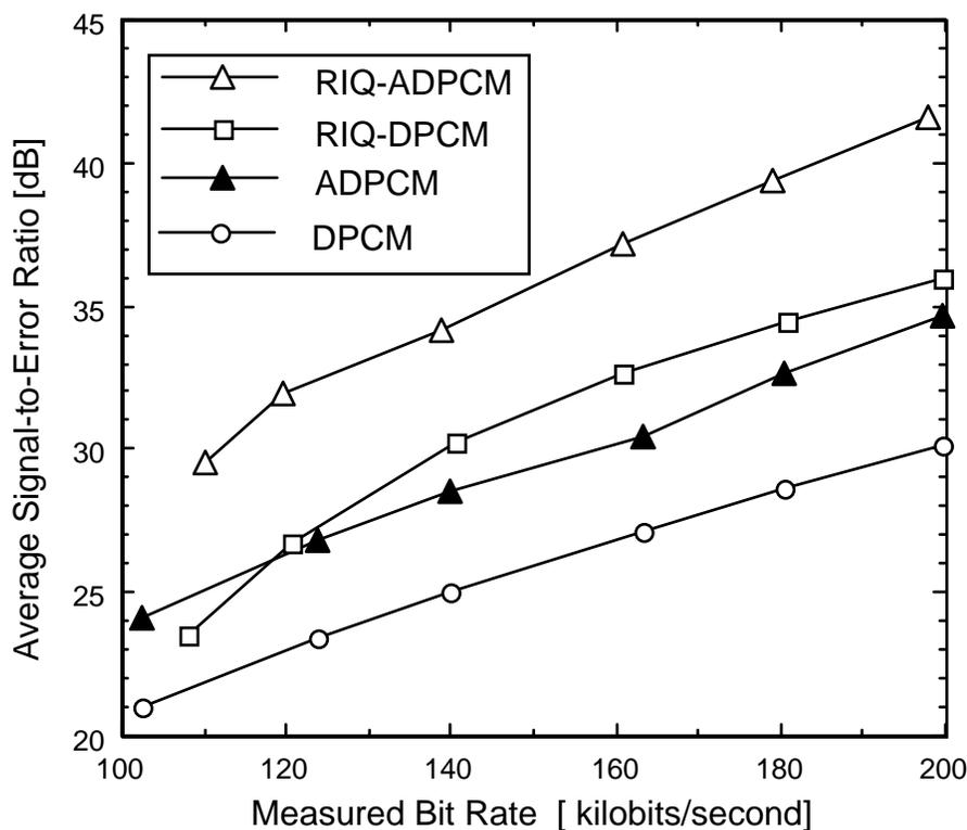
**Figure 2:** Simulation results and performance comparison of DPCM, DPCM with adaptive quantization, RIQ-DPCM, and RIQ-DPCM with adaptive quantization.
