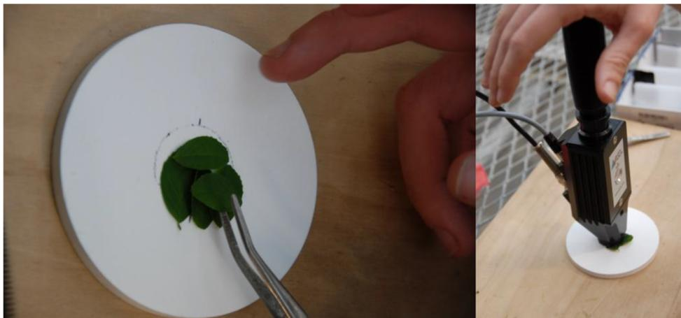
**Figure 3. Sampling method.** Two dissected alfalfa leaves on the spectralon target (left). The ASD fiber optic and plant probe assembly (right).
